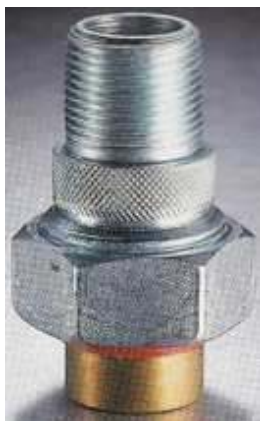
Lead Free Brass Dielectric Union Male Iron Pipe Thread X Sweat
